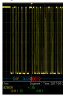
Segmented is a unique mode that specifically captures pulses, rare events, or infrequent glitches. Capturing the downtime between infrequent events in normal acquisition mode wastes memory. With segmented memory, you can eliminate that time and focus on the portions of the signal you want to analyze in greater detail.
