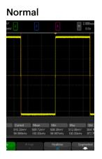
Normal is the most used mode for day-to-day measurements. This mode acquires samples at a specified sample rate and displays them on the screen at each trigger event. This mode is the safest to use.
