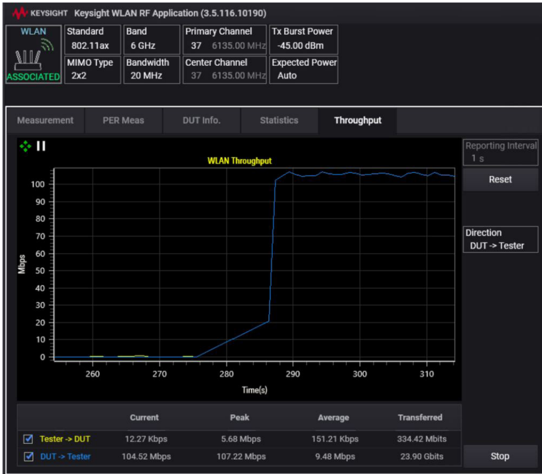
Figure 6. Wi-Fi throughput testing with the E7515W UXM wireless connectivity test platform
