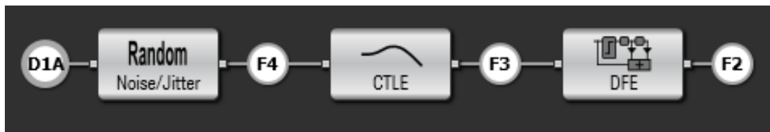
Figure 9. Reference receiver noise and equalizer components
