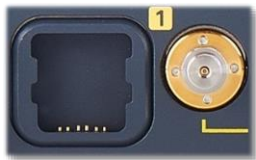
Ruggedized 1 mm Male Bulkhead Connector with AutoProbe III Interface
