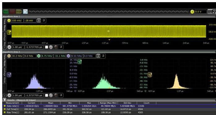
With its flat frequency response and low noise, the UXR-Series can measure jitter components such as ISI.
