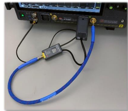
PrecisionProbe characterization of a 1.85 mm cable to 70 GHz using the N2126A calibration module
