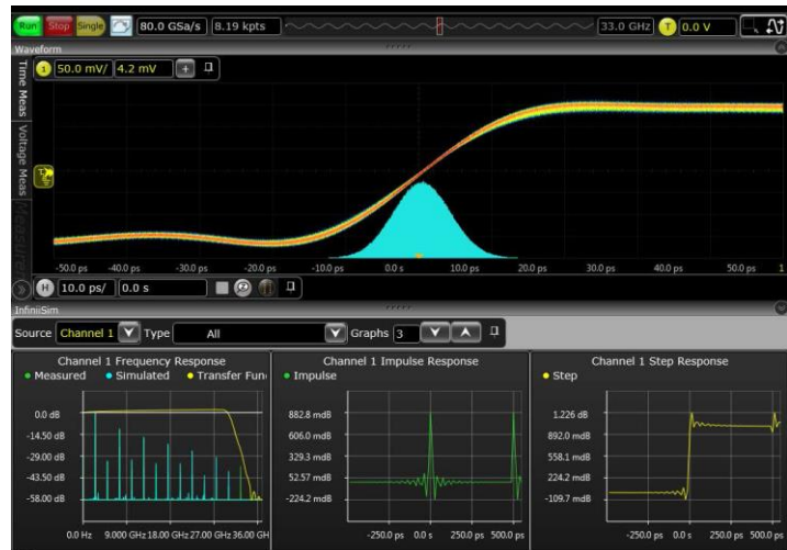
InfiniiSim renders the waveform through hardware acceleration
