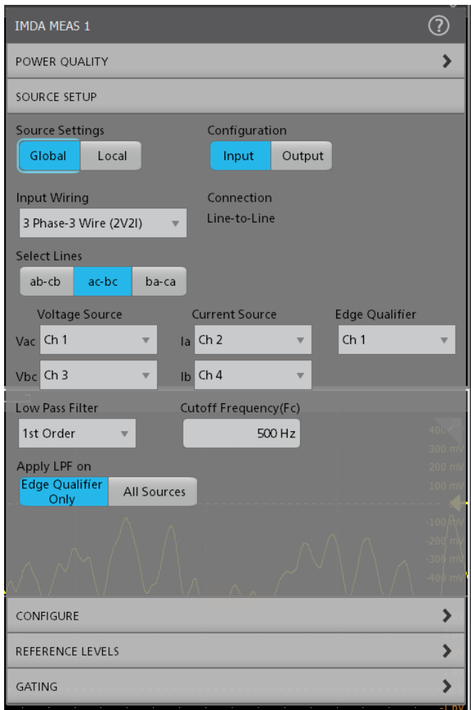
Figure 16. Setup for a 3-wire system using the two-wattmeter method. Currents are measured on phases A and B, with voltages on phases A and B measured with respect to phase C.
