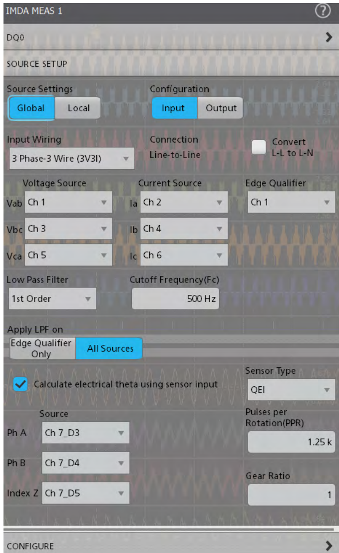
Figure 28. Configuring the oscilloscope for DQ0 measurements on a system using a quadrature encoder interface (QEI).
