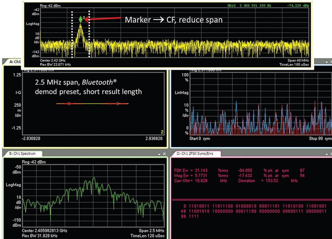
**Figure 18.** By selecting a portion of the capture bugger, reducing frequency span, and changing the center frequency to match (top), post-processing in the 89600 VSA provides isolation and analysis of any signal in the capture bugger including demodulation of this single Bluetooth hop (bottom).
