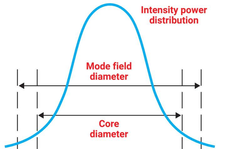
Figure 3. Mode field diameter concept
