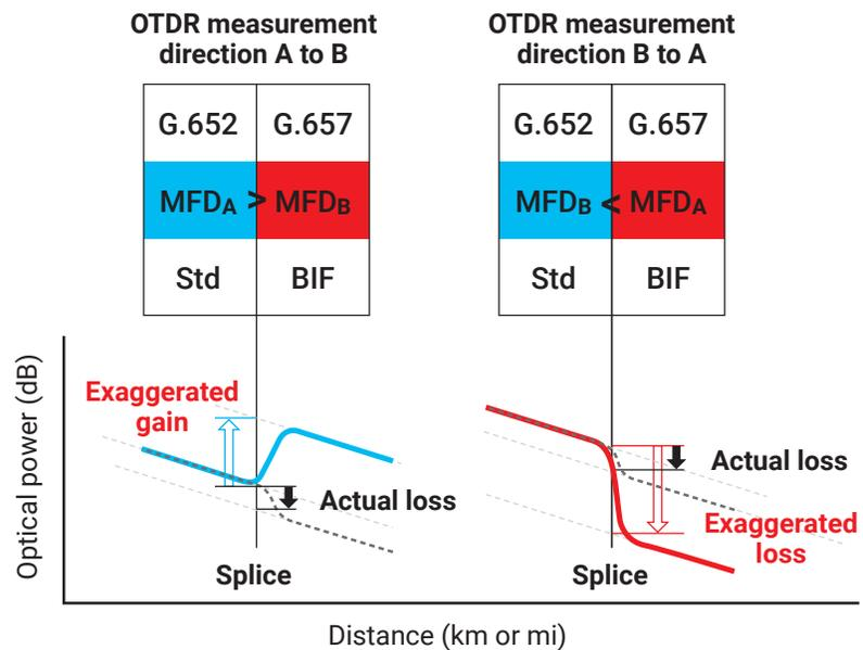
Figure 4. Exaggerated gain and loss due to MFD discontinuity (Courtesy of Corning)
