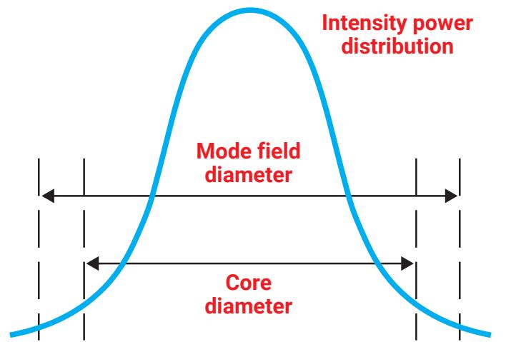
Figure 3. Mode field diameter concept
