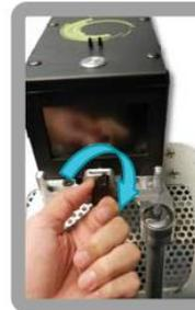
4 Once AIR Mount is secured onto antenna, install RF Aligner on mounting plate and tighten knob to secure the Aligner.
