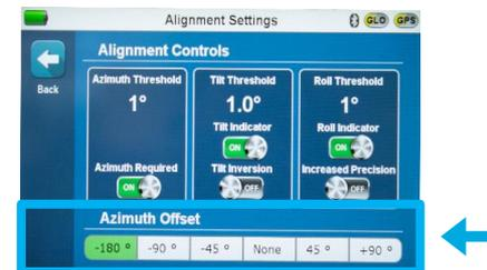
If RF Vision is installed with an offset, Navigate to Alignment settings and set associated offset.
