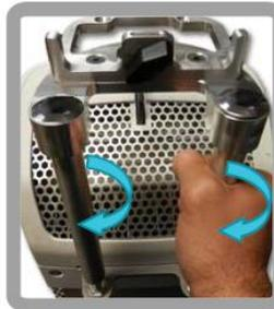
3 Turn posts simultaneously so that they thread evenly onto M60 bolts.
