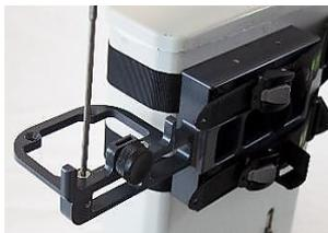
Remove M6 bolts from mounting plate to reconfigure bracket.
