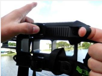
Remove ladder straps from ratchet buckles by lifting up on the release latch and pulling back on the loop.
