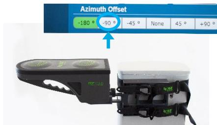
Install RF Vision, adjust offset in "Alignment Settings" and perform measurement.
