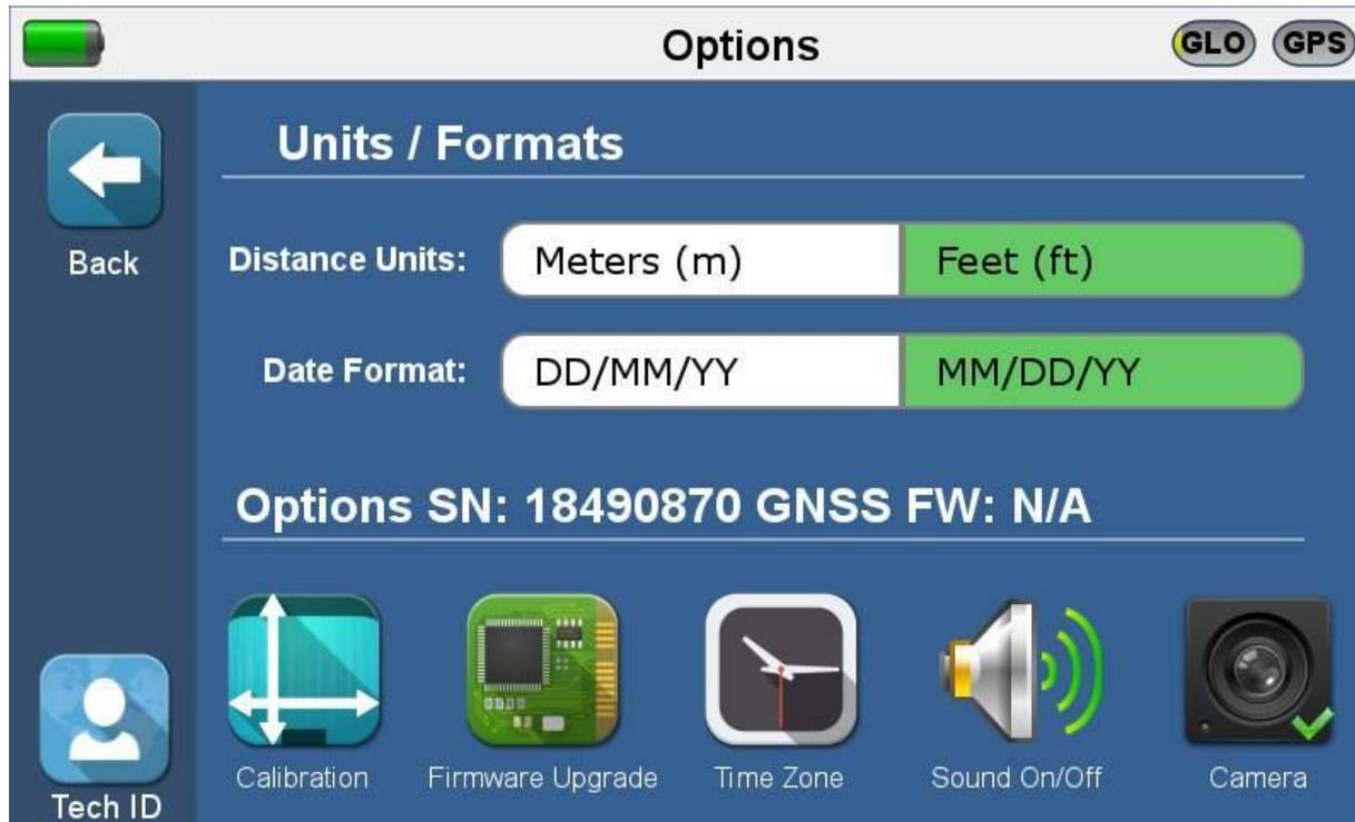
Select units / formats, perform tilt calibration, upgrade the firmware, set the time zone, turn the sound on/off, and set up the RF Vision camera license.
