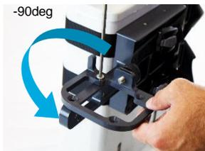
Rotate the mounting plate to desired offset (i.e. -90deg).
