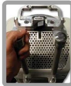
2 Line up AIR Mount vertical posts with existing M60 bolts.
