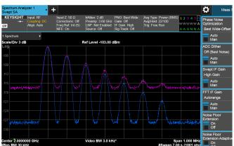
Accurately measure low-level signals to reduce measurement noise by up to 10 dB with Noise Floor Extension (NFE).
