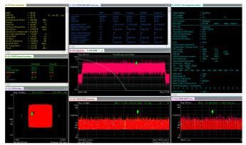
Use 89600 PathWave VSA software to gain deeper insights of DOCSIS 3.1 downstream signals through MER/BER summaries, PLC decoding information, and peak MER traces on the constellation, subcarrier and symbol domains.
