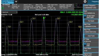
Simplify complex tasks using limit lines and built-in distortion analysis measurements.
