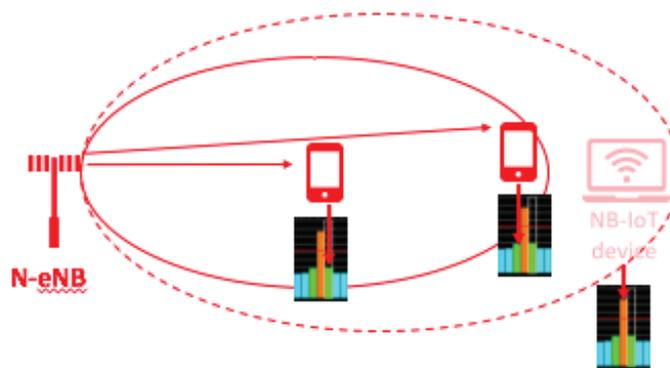
Figure 17 - Effect of NB-IoT power boosting on adjacent PRBs from the same cell site
