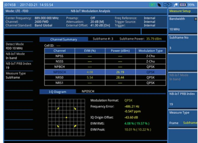
Figure 12 - Subframe #1/2/3/4 measuring NPDSCH(S)CH
