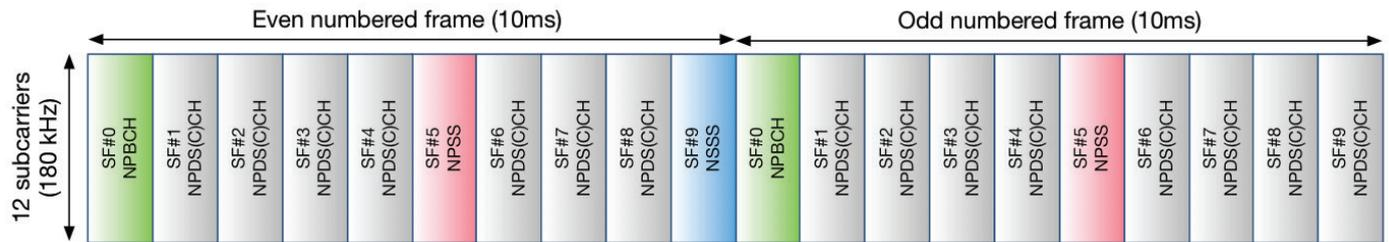
Figure 10 - NB-IoT Frame Structure. Note physical channels and signals are primarily multiplexed in time.
