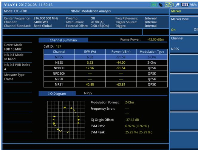
Figure 13 - Subframe #5 measuring NPSS
