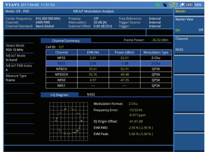
Figure 14 - Subframe #9 measuring NSSS (when available)
