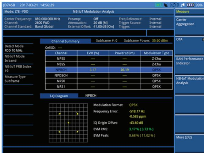
Figure 11 - Subframe #0 measuring NPBCH
