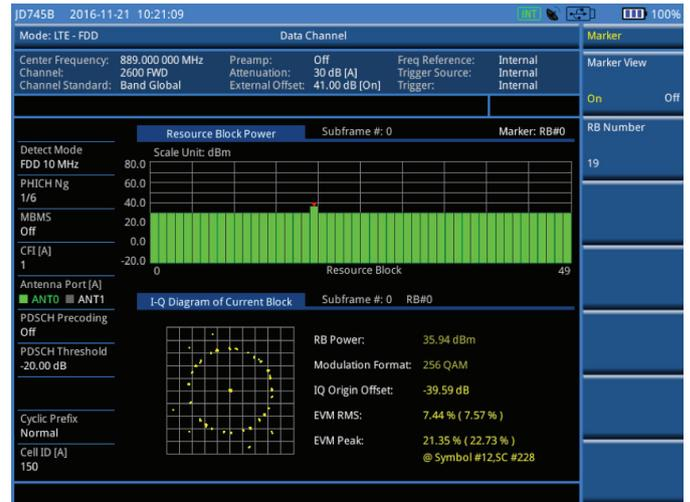
Figure 8 - LTE Data Channels (PDSCH)
