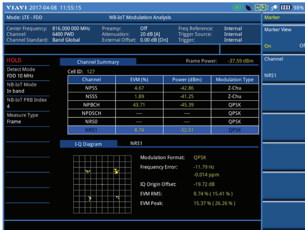
Figure 9 - NB-IoT (in-band) Signal Quality and Modulation Analysis
