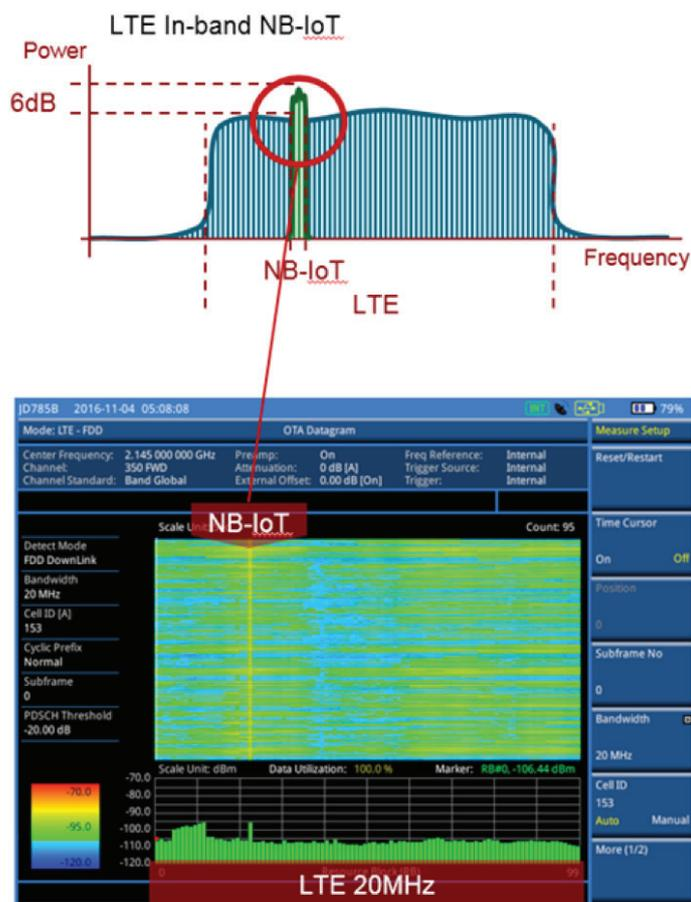
Figure 5 - Datagram view for LTE & NB-IoT (in-band) downlink PRBs
