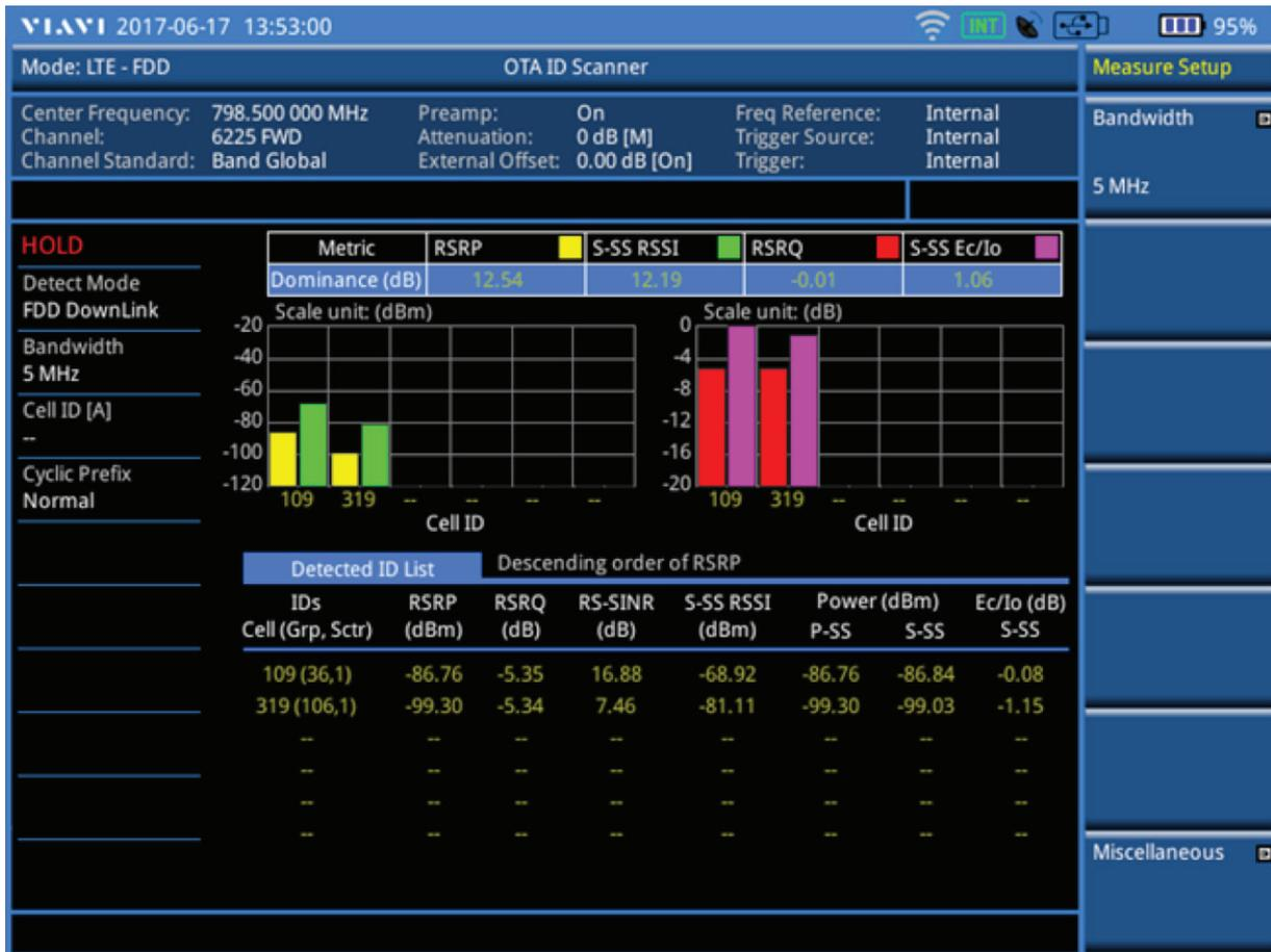
Figure 4 - Example channel analysis for Cell IDs #109 and #319
