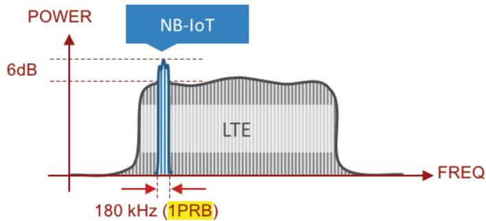
Fig.1 NB-IoT in-band operation
