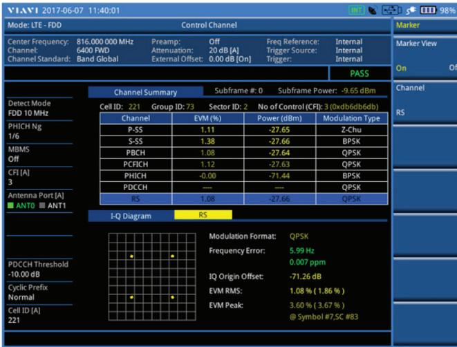
Figure 7 - LTE Control Channels
