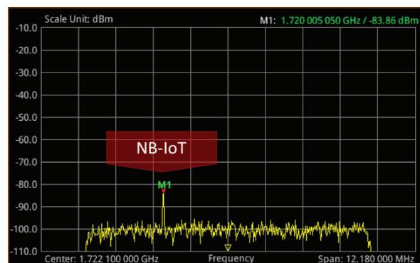
Note the downlink capture above shows the LTE signal with both Max and Min Hold averages, a very convenient form of visualizing the maximum and minimum values of a real-life LTE signal through time.
